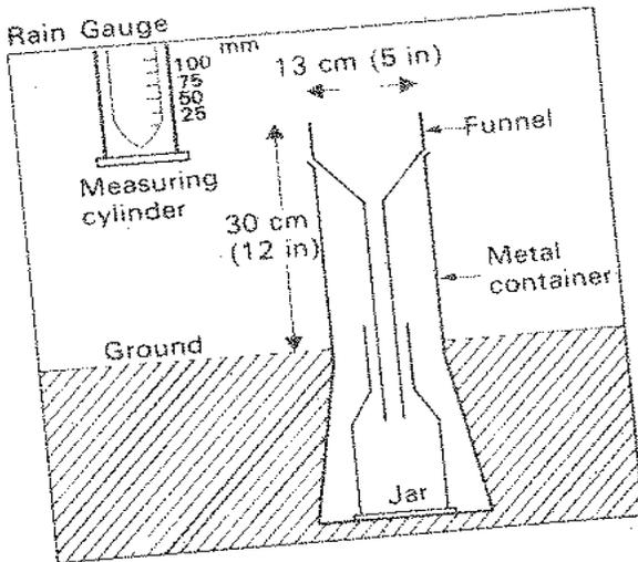
**Positioning of a rain gauge at a weather station.**
